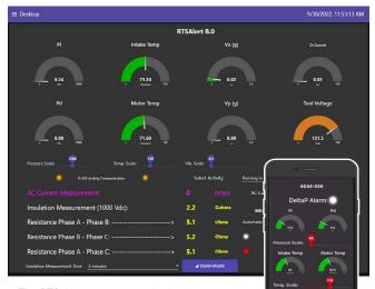
The RTS Alert continuous deployment monitoring system provides visual surveillance of key parameters via Bluetooth-connected mobile and tablet devices.
